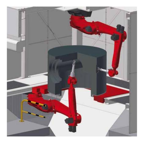
The benchmark **PRIMUSS** innovation integrates the highest level of automation and control technology in the design and manufacture of monolithic manhole bases with bespoke mixed inlet and outlet entries and benching. In using proven robotic programming the varying location, diameter and angular dimensions of different pipe inlets permit precise milling by **PRIMUSS** immediately after product demoulding.
